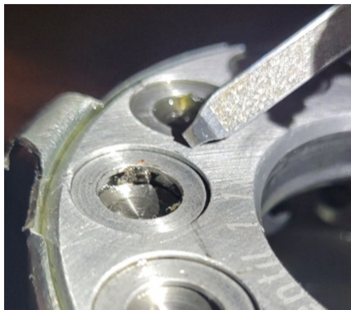
Bypass valve held open by debris, preventing proper sealing.
